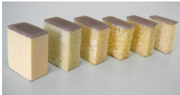
Figure 1. Models of trabecular bone used in the experiments. From left to right: 123-MPa solid-and-rigid polyurethane-foam block; 137-, 47.5-, 23-, and 12.4-MPa closed-cell blocks; and 6.5-MPa open-cell block. All blocks had 2-mm-thick cortex attached.
